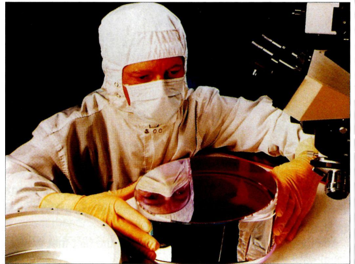
One of the LIGO mirrors which achieves parts-per-million losses.
